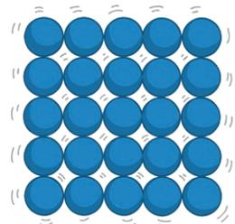
The particles in a **solid** are arranged in a regular pattern. The particles in a solid **vibrate** in a fixed position and are tightly packed together. The particles in a solid have a **low amount of kinetic energy**.
