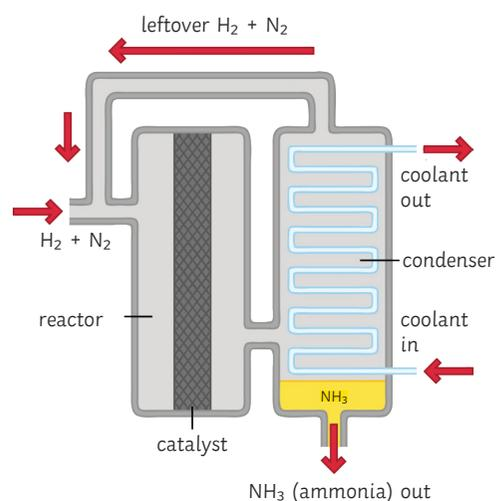
The Haber process is used by the chemical industry to synthesise **ammonia**. Ammonia is used in the production of fertilisers, dyes and explosives.
